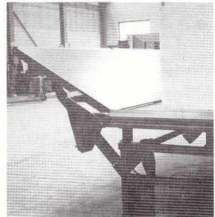
Restplate outside with motorized tilt and rise.
