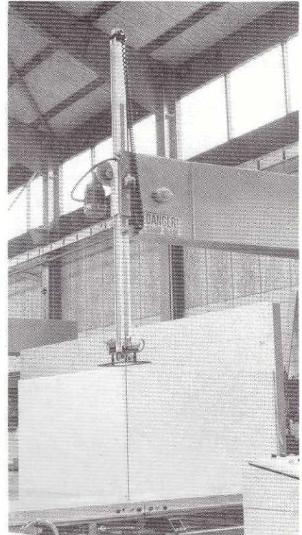
Motorized height-adjustment of blade guard.
