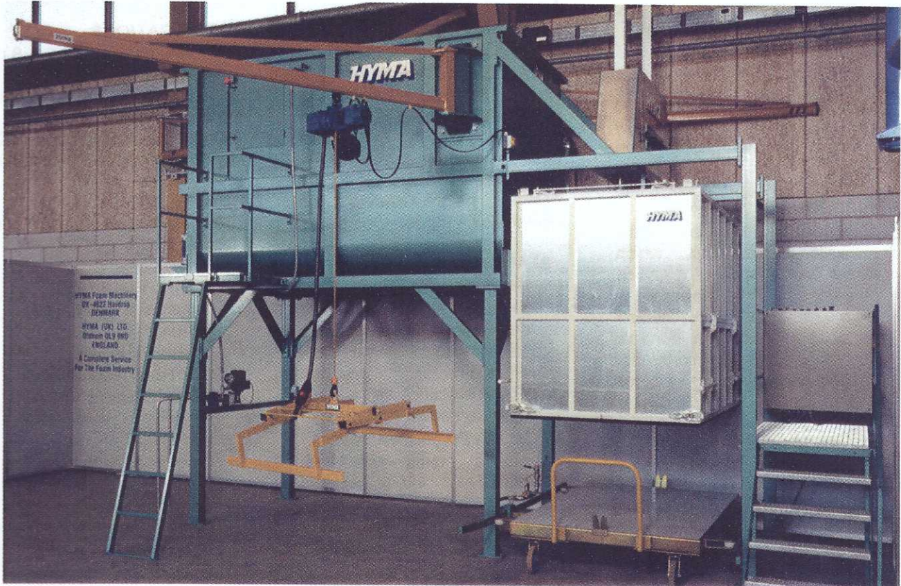
Module built Chip-Foam Plant Type BFE for environmental friendly recycling of PU scrap foam
