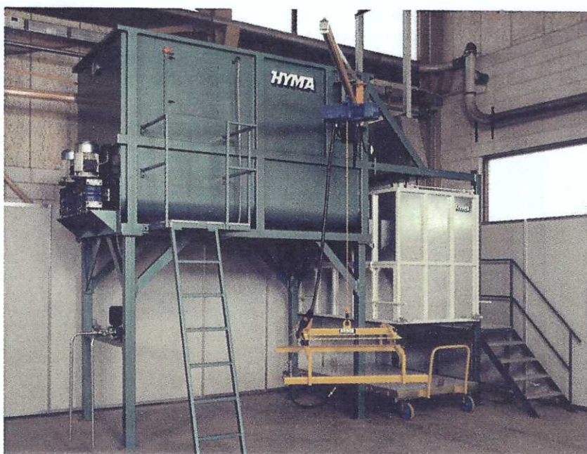
Chip-Foam Plant Type BFE with steam-cure system
