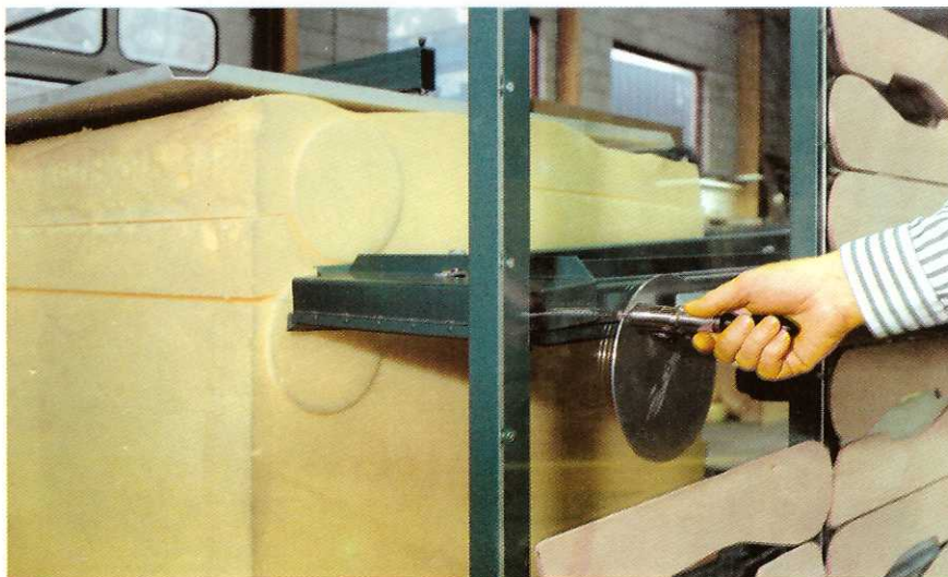
Template for guiding the cutting wire to cut required shape.
