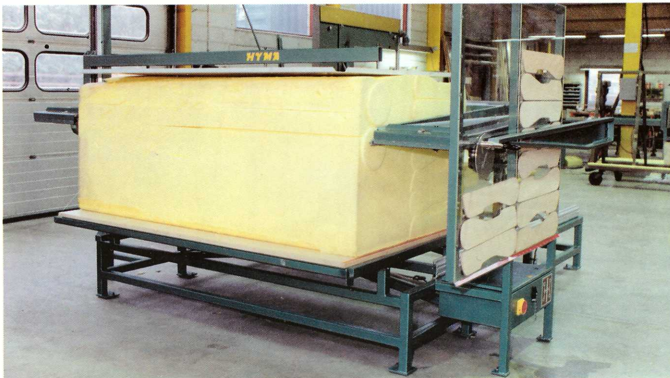
The HYMA Manual Contour Cutting Machine Type CCM-210
