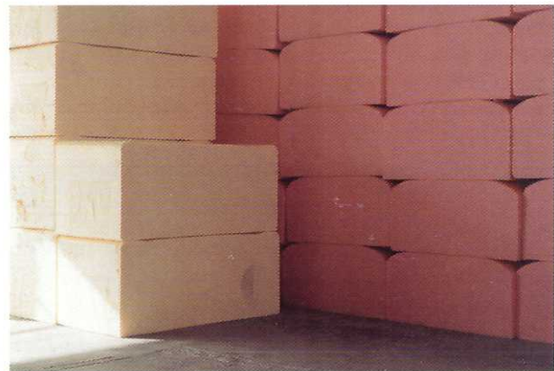
On the left, Foam blocks from Flat-top machine; on right domed blocks from conventional machine.
