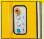
The machine has a repeat The machine has a repeat function, which increases the compression of the material. It can be activated by pressing the button in the middle on the control panel.
