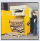
Automatic discharge onto pallet The compacted bales are ejec-ted automatically onto the pallet using a safe two-handed opera-tion. In addition, the machine can be locked to prevent unauthorised access.
