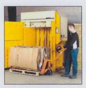
Easy after-handling The compacted bales can sub-sequently be stacked anywhere requiring only a minimum of space until they are picked up. The bales are bound either by plastic strap or steel wire.
