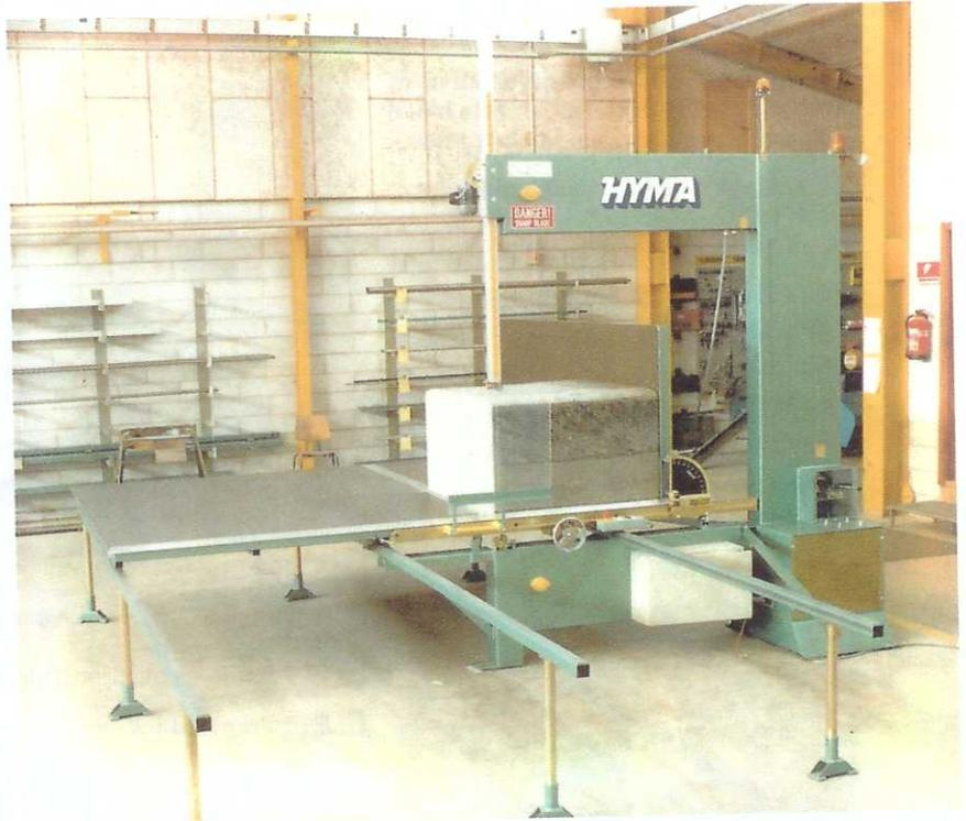
The NSL Vertical Cutting Machine with coated table.
