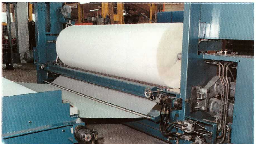
Peeling of Foam Foil on the RSS Machine with Rewinding unit.
