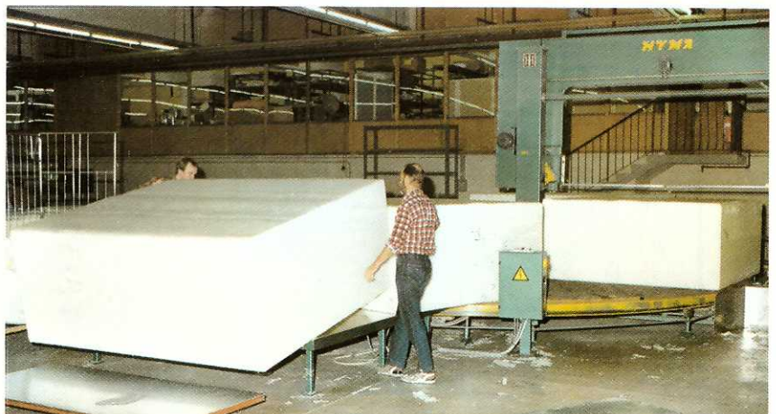
Easy loading and unloading of blocks with airfloatation table
