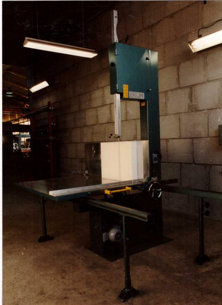
Type SLM is the smallest Vertical Cutting Machine in our programme. It is a two-wheel machine, thus the inside cutting width is limited by the diameter of the knife wheels.
