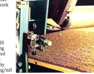
SSB-H cutting bonded foam density 450 kg/m3
