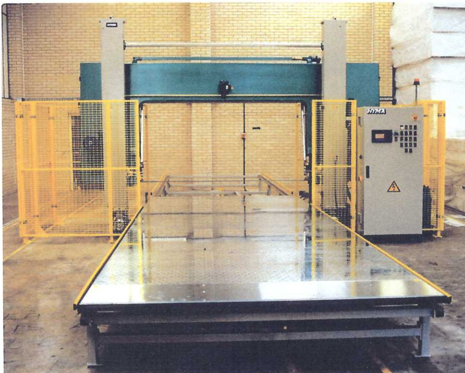
Horizontal Stack Slitter SSH with 4,2 m table.
