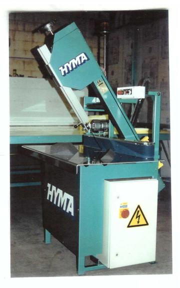
The HYMA Type VSM cutting machine is an alternative to the full size production machine, particulary when only limited numbers of special and smaller forms are required.
